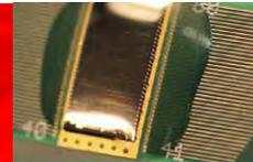
Silicon nitride photonic integrated circuit
